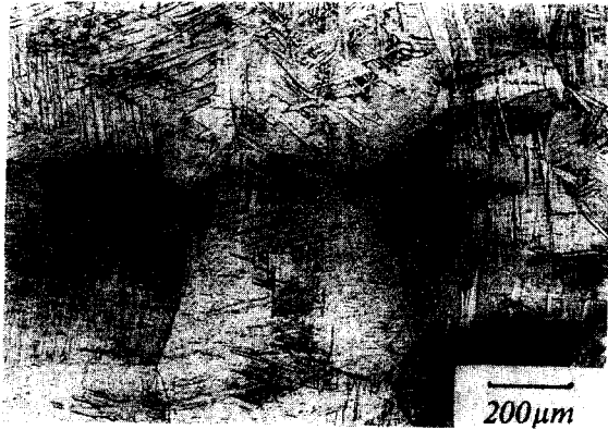
Fig. 4. Optical micrograph of structure of treated Ti-6Al-4V alloy.
