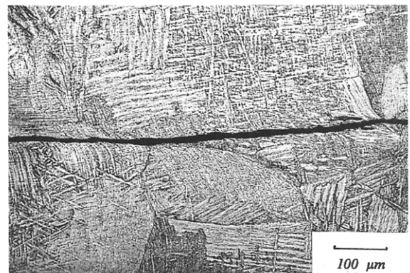
Fig. 9. Coalescence of microcracks in localized zone.
